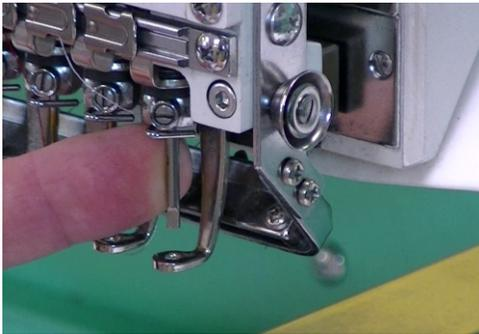
Remove the needle that is currently in position over the Lower Arm. Replace it with one of the RhAT tools. The Flat on the bottom of the RhAT tool should face the front of the machine. The Notch at the bottom of the tool should face the back.
