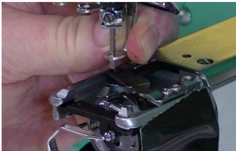
Grip the back of the Presser Foot as shown and push it up. The RhAT tool should slide easily through the hole in the Presser Foot. If the hole is too small, stop and see the notice at the end of this instruction sheet. If the presser foot has been bent from striking a hoop or other object, the RhAT tool may be deflected when making the adjustment.
