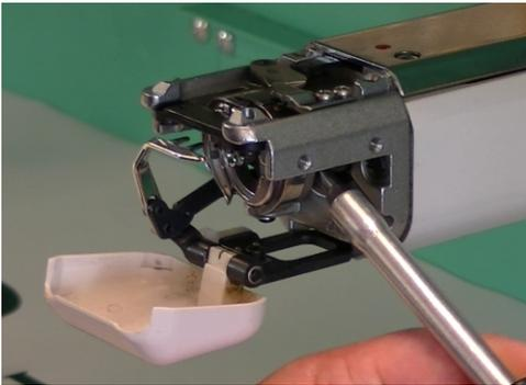
At 160 degrees, you can loosen the other recessed screw in the Rotary Hook.
