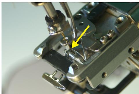
**CHECK YOUR WORK.** The point of the Rotary Hook should be directly behind the Needle. The gap should be just large enough for a thread to go through. A gap that is too wide will cause looping and missed stitches. A gap that is too narrow will result in numerous thread breaks. That is why there are five tools included with the set.
