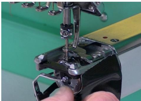
If you are at the correct setting position, remove the tape that has been keeping the Rotary Hook from moving.
