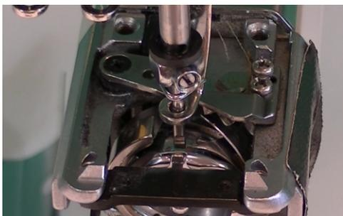
After rotating the Main Shaft to 182 degrees, the tip of the RhAT tool will be about .090" above the basket of the Bobbin and centered in the gap. The point of the Rotary Hook should still be about 1/8" to the right of the RhAT tool.
