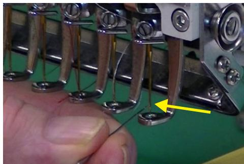
Included in the RhAT set is a Cylindrical Magnet. Use it to verify that the grooves in all of your Needles are aligned.
