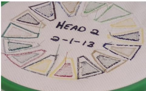
Thread should be tight on top and only have about 1/3 of the Bobbin thread showing underneath. If some colors or needles sew better than others, check your tensions. You should invest in a Upper Thread Tension Gage and use it whenever you change threads. Tension should always be the first thing to check when loose stitching is encountered.
