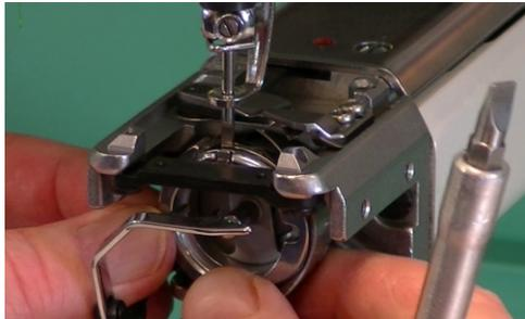
*You should be able to make the RhAT and the Needle Bar deflect by rotating the Rotary Hook counter-clockwise or by pulling it forward. Even a slight pressure on the Rotary Hook should make it move.*
