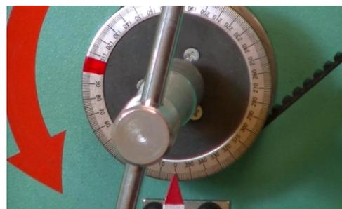
If the tip of the RhAT tool is above the tip on the Rotary Hook, turn the Main Shaft to 0 degrees (or the Upper Dead Point).
