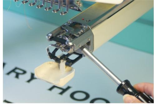
Rotate the Main Shaft using your T-Handle in the correct direction (counterclock-wise on the TMFX) until the pointer is at 160 degrees.
