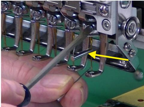
Place the Magnet on the front of each Needle across this groove and it will indicate whether it is straight or not. If it is at an angle, correct it. A rotated Needle will cause frayed and broken thread, as it will affect the timing and clearance of the Rotary Hook. Check your Needles whenever you change them.
