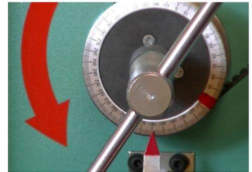
Tighten the one accessible screw.
