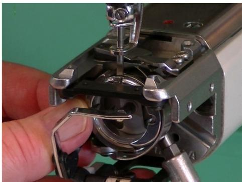
While holding the Rotary Hook in position with your left hand, tighten the protruding screw on the Rotary Hook. Check your work.
