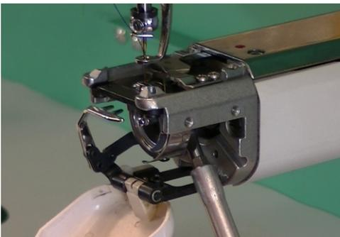
With the Degree Wheel at about 200 degrees, you can now loosen the protruding screw on the Rotary Hook.
