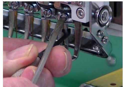
Proper alignment is important. The flat at the bottom of the Tool should be parallel to the frame of the machine. Make sure the RhAT tool is as far up into the needle bar as it will go.
