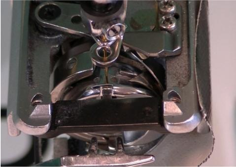
The needle is shown here properly centered in the gap. The Rotary Hook is taped to the arm.
