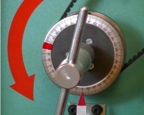
Rotate the Main Shaft to 0 degrees.
