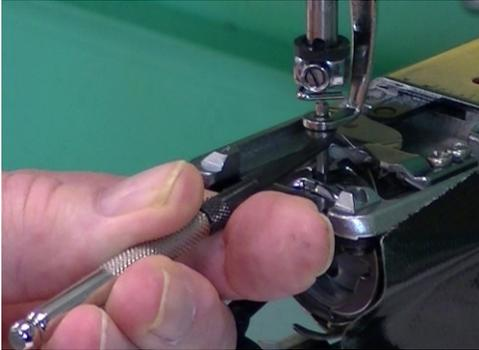
While holding up on the Wrench, loosen the needle retention screw and let the RhAT tool slide down until it rests on the bottom of the Bobbin basket. Retighten the Screw holding the RhAT tool (do not over tighten the screw) and remove the Wrench.
