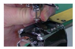
Grip the back of the Presser Foot as shown and push it up. The RhAT tool should slide easily through the hole in the Presser Foot. If the hole is to small, stop and see the notice at the end of this instruction sheet. If the presser foot has been bent from striking a hoop or other object, The RhAT tool may be deflected when making the adjustment.
