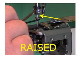
Verify that the tip of the RhAT tool is above the tip on the Rotary Hook. If for some reason it will not clear, loosen the protruding screw on the Rotary Hook, recenter the tool in the gap, secure the Rotary Hook with tape again before returning the main shaft to 0 degrees (or Upper Dead Point).
