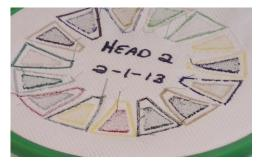
Thread should be tight on top and only have about 1/3 of the Bobbin thread showing underneath. If some colors or needles sew better than others, check your tensions. You should invest in a Upper Thread Tension Gage and use it whenever you change threads. Tension should always be the first thing to check when loose stitching in encountered.
