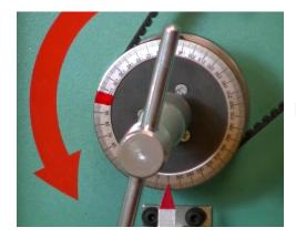
Rotate the Main Shaft to 0 degrees.
