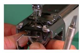
You should be able to make the RhAT and the Needle Bar deflect by rotating the Rotary Hook counter-clockwise or by pulling it forward. Even a slight pressure on the Rotary Hook should make it move.
