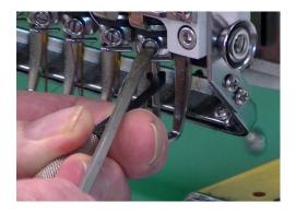
Proper alignment is important. The flat at the bottom of the Tool should be parallel to the frame of the machine. Make sure the RhAT tool is as far up into the needle bar as it will go.
