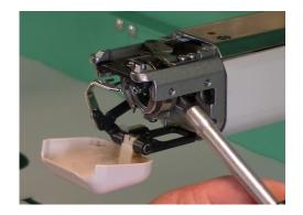
At 160 degrees, you can loosen the other recessed screw in the Rotary Hook.
