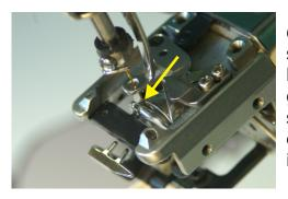
**CHECK YOUR WORK**. The point of the Rotary Hook should be directly behind the Needle. The gap should be just large enough for a thread to go through. A gap that is too wide will cause looping and missed stitches. A gap that is too narrow will result in numerous thread breaks. That is why there are five tools included with the set.
