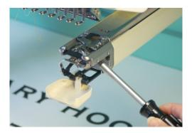
Rotate the Main Shaft using your T-Handle in the correct direction (counterclock-wise on the TMFX) until the pointer is at 160 degrees.
