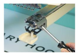
Reinstall the U Shaped Cover and the Needle Plate. Replace the Bobbin. Rotate the Main Shaft back into the Red Zone. Restart the Machine.
