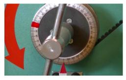
If the tip of the RhAT tool is above the tip on the Rotary Hook, turn the Main Shaft to 0 degrees (or the Upper Dead Point).
