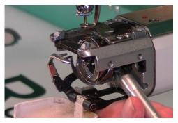
Tighten the one accessible screw.
