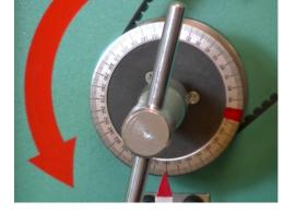
While turning the Main Shaft to 182 degrees, the RhAT tool should come all the way down and start back up. You may not be able to see the movement as it starts back up. It should not make contact with the Rotary Hook. You might want to have someone watch for interference the first time you use the tool on your machine.
