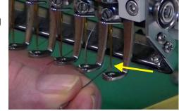
Included in the RhAT set is a Cylindrical Magnet. Use it to verify that the grooves in all of your Needles are aligned.
