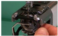
Be careful to NOT EXERT pressure that will deflect the RhAt and/or the Needle bar. If you see the RhAT and the Needle Bar shift or deflect, either to the left or forward, you are pushing to hard and your adjustment will be wrong.
